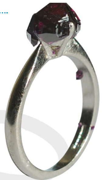
A researcher at the University of the West of England has created the first lab-grown ruby in situ. The material was developed within a platinum ring. Photo by Sophie Boons.
